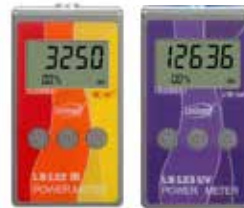
IR & UV Meters Capture glass performance - use pre and post-application.
